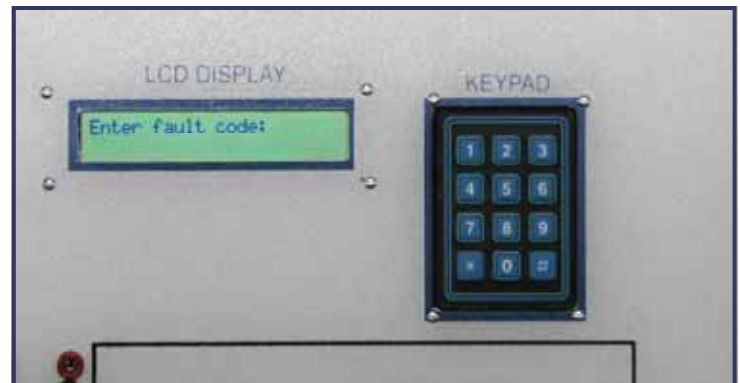
Student Response and Local Fault Insertion Panel
