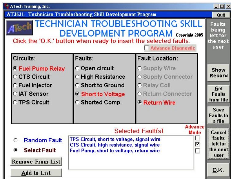
Figure 2 - Leaving Faults for the Next User
