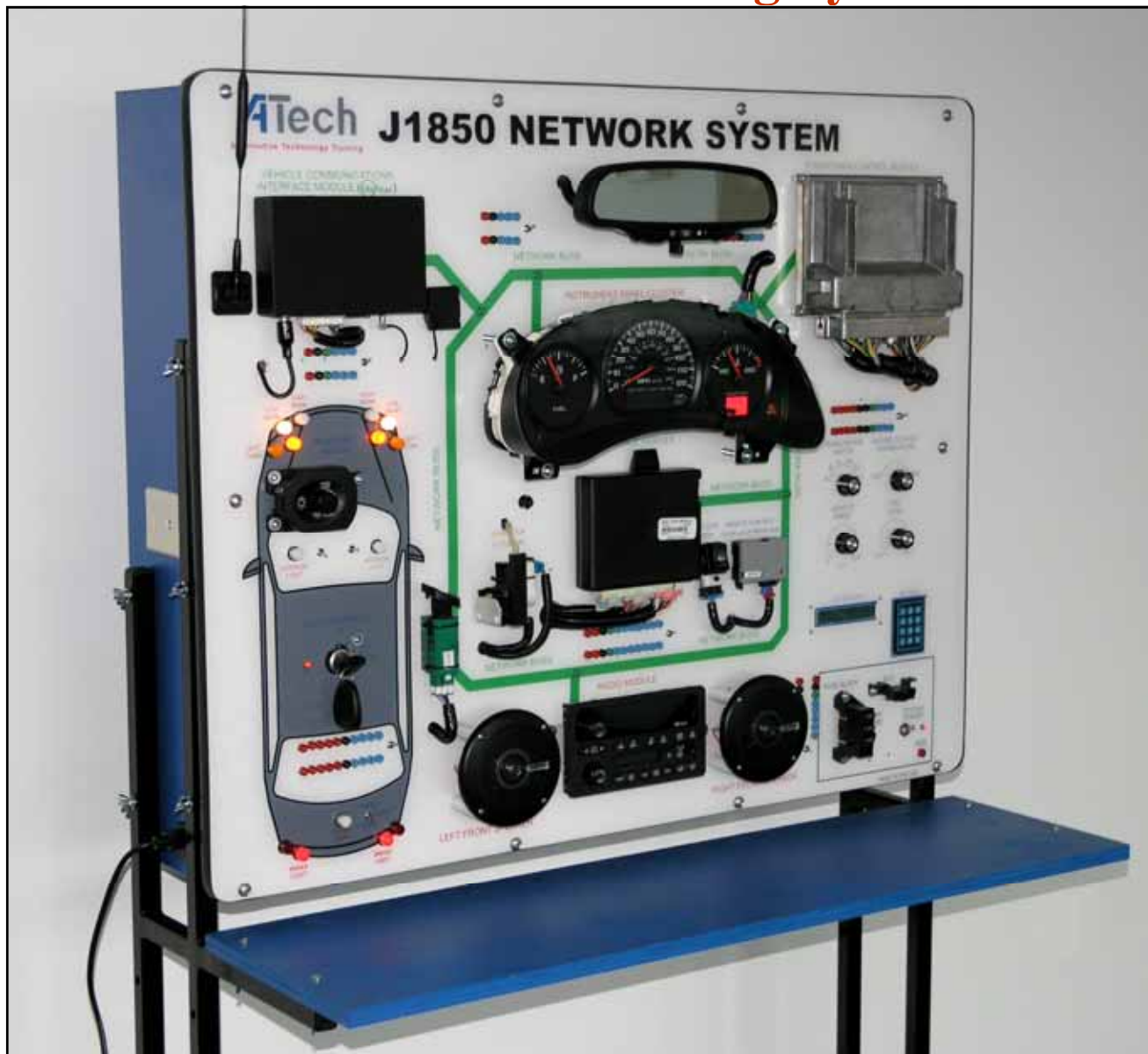
3801 J1850 Network Training System (floor model configuration)
