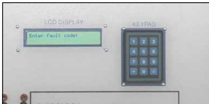
Student Response and Local Fault Insertion Panel
