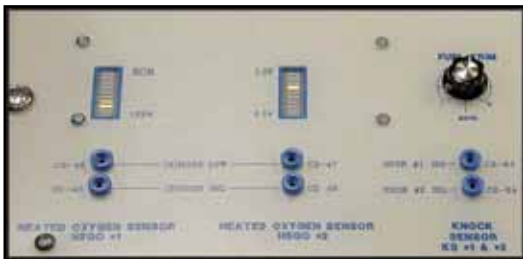
Oxygen Sensors and Fuel Trim Control
